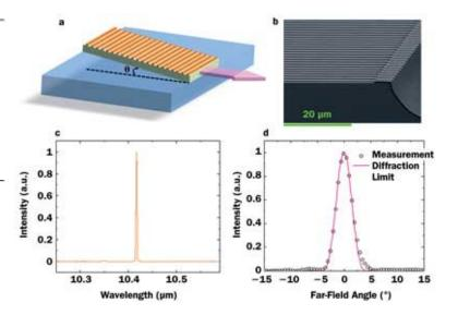
a new type of distributed feedback mechanism called B-DFB, a simple diffractive feedback in an angled laser cavity.
